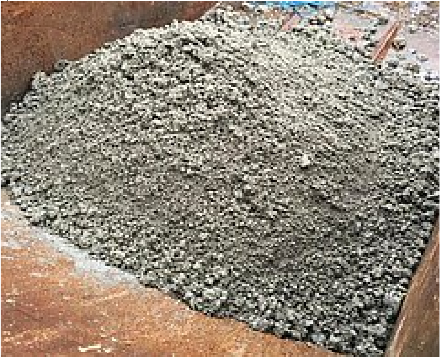
Dewatered sludge cake from the Q-PRESS®
