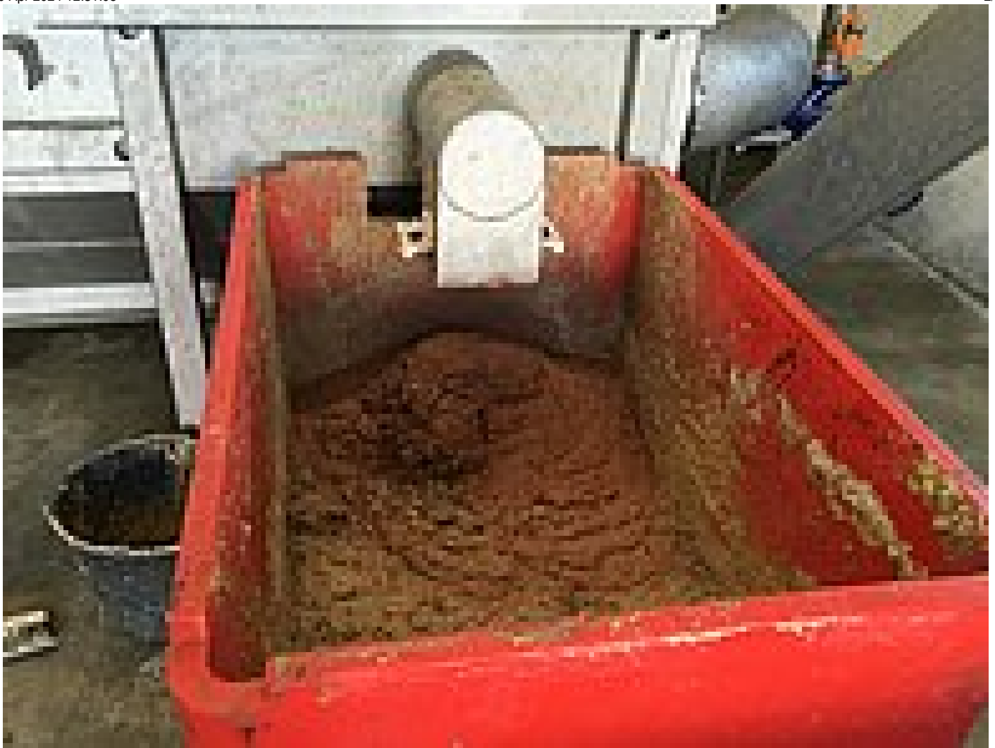
Discharge from the fat separation
