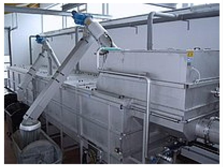
For reasons of operational safety the first step of sewage treatment works is generally mechanical wastewater pre-treatment to prevent operational problems, such as blockages, wear, or silting.
